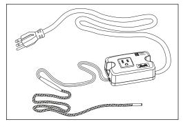
The RX1200 controller is designed to use in conjunction with Danfoss roof and gutter de-icing cable for roof, gutter and snow melting applications. The RX1200 sense both moisture and temperature conditions in the gutter or downspouts and turns the roof de-icing cable on and off based upon these readings. By combining the moisture and temperature readings, the controller is able to save up to 75% on energy consumption compared to a controller which only measure temperature.
