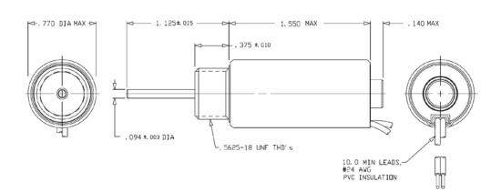
Solenoid shown energized with plunger fully seated Supplied with hex nut shipped loose Spring kits available (consult factory)
