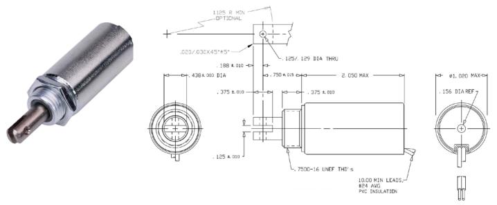
Solenoid shown energized with plunger fully seated Supplied with hex nut shipped loose Spring kits available (consult factory)
