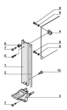
Plug in unit, front anodized, rear etched, shielded (textile), front assembly... http://schroff.pentair.com/SpecificationSheetDisplay?catalogId=307445...
