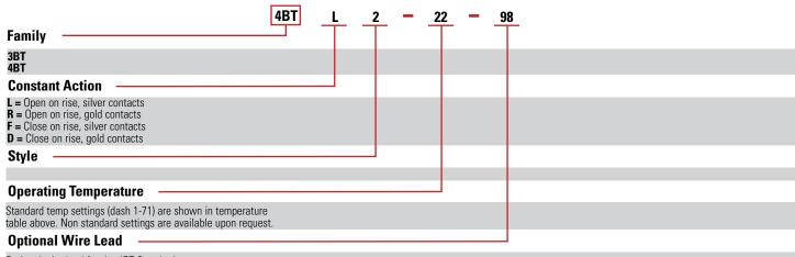
Optional wire lead for the 4BT Standard: **98** = 12" stranded 22 gauge white Teflon insulated (omit if leads are not required).
