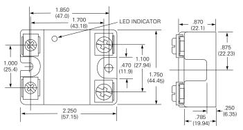
Dimensions are in inches over (millimeters) unless otherwise specified.
