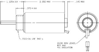
Solenoid shown energized with plunger fully seated Supplied with hex nut shipped loose Spring kits available (consult factory)
